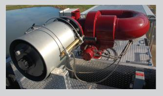
Williams Fire & Hazard Ranger 3 Plus with flows up to 4000 GPM or the Williams Ambassador 1x4 with flows up to 6000 GPM. Both are available with radio remote controls, as well as a Hydro-Chem nozzle for 3 dimensional fires.
