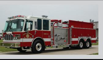
Inundator industrial foam tanker apparatus from Ferrara are heavy duty trucks designed to be used as a pumper or as a foam supply unit, with tank size available from 1500 to 3000 gallons.
