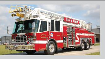
Ferrara has a complete lineup of industrial aerial apparatus. We offer the SHD-100, a super heavy duty, 3-section aerial ladder with a 100' vertical reach. The aerial can flow up to 2000 GPM.
