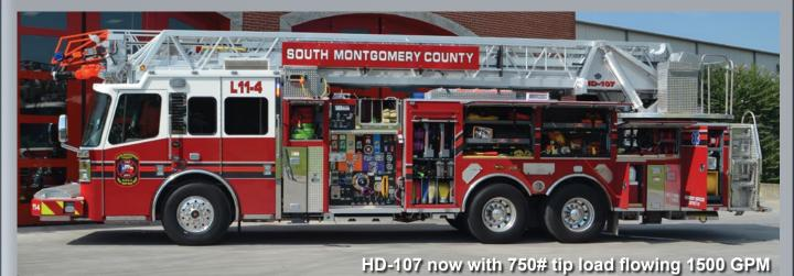
HD-107 Aerial Ladder, 2000 GPM pump, 200 CFM CAFS, full ISO ground ladders, hose and equipment, 225" wheelbase
