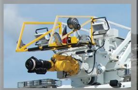
Move the monitor from tip to lower section with the flip of a switch
