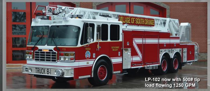
Each Ferrara Ladder is available in a low profile design. The HD-100 mid mount has a travel height as low as 9'10". If you need a rear mount, the LP-102 is available under 10'4", the HD-77 as low as 10'4", and the HD-107 as low as 11'4". Check out the FD-100, 2-jack rear mount aerial ladder at 10'10".
