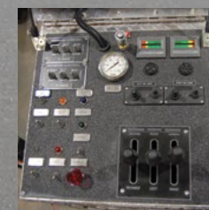
Turntable control console has direct hydraulic controls
