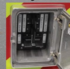
Outriggers have large paddle controls, easy to use with a gloved hand
