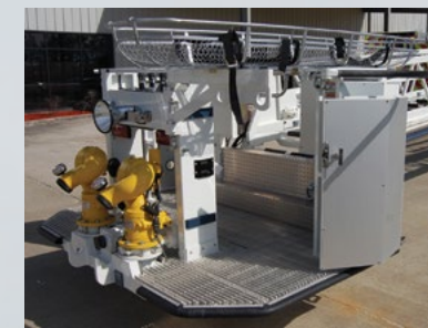
500 pound rappelling arm doubles as a stokes basket mount with tie down strap and cleats
