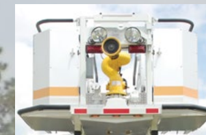
Full 180 degree horizontal nozzle movement flowing at 1500 GPM
