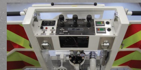
Platform control panel is located front and center, including shift on the fly speed controls
