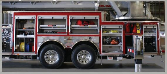
Over 200 cubic feet of storage space as a Quint. Over 525 cubic feet with no pump-no tank
