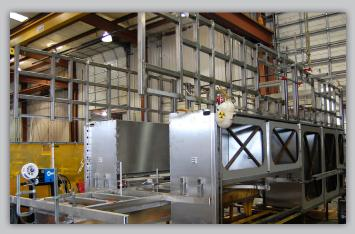
The upper body is framed with welded stainless steel tubing and then overlaid with 12 gauge stainless steel plate. This upper body structure gives the body dditional strength and also creates a safe interior for crews to do their work.
