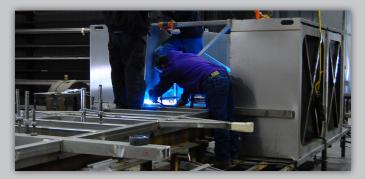
The strength of the stainless steel body starts with the subframe. Constructed from welded stainless steel tube, flat bar, angle and plate, this structure supports the entire body. The primary shape in the subframe is a 2" x 3" x 3/8" thick stainless steel tube, used for full width crossmembers and floor joists.
