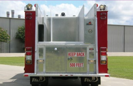
If hose bed height is a concern, use our optional low hose bed configuration with a 500, 750 or 1000 gallon tank.
