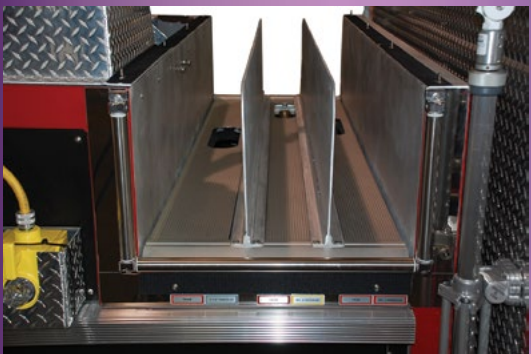
We build crosslays with the attention to detail you expect from Ferrara. Adjustable dividers, full width ribbed flooring, stainless steel trim plates and 3-way rollers are all standard equipment.
