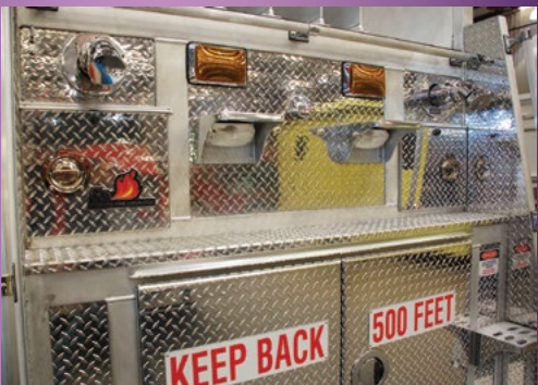
Cast, non slip steps with integral lights are standard, along with raised surface handrails
