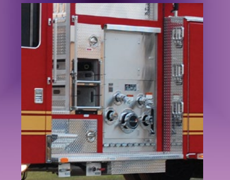
Speedlays have the same features as our crosslays and are available with top, side or rear mount pump panels.
