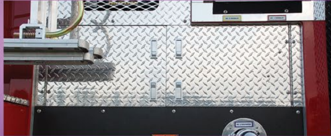
Side panel trucks have a large, right side pump access panel. Top mounts have this on left and right sides.
