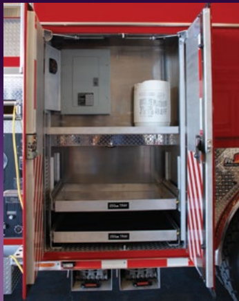
Our 3/16" thick aluminum compartments are built to carry all the equipment you need. They are standard with a 25" deep lower area and 12" deep high sides.
