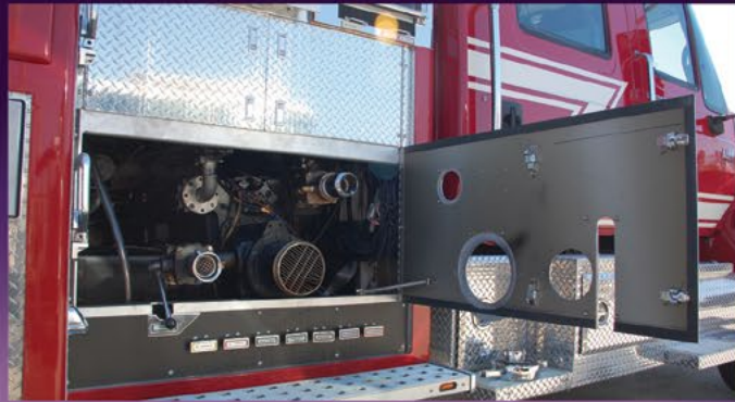
Improve service access with our optional hinged pump panel. Simply remove caps and elbows to open the entire panel.
