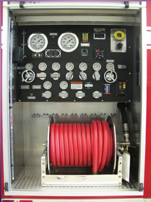
Our budget and service friendly rear mount pump installation allows you to use manual valve actuators in an easy to read panel.
