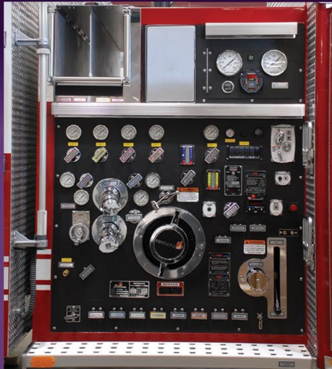
Black anodized aluminum pump panels are non glare and easy for the pump operator to use.
