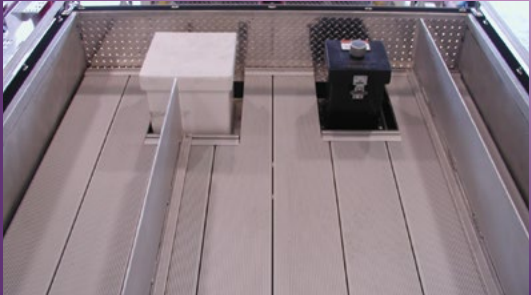
The hose bed is made from 3" x 3.5" and 2" x 4" tubular extrusions, slotted to receive 3/16" thick 5052 H-32 marine grade aluminum plate.
