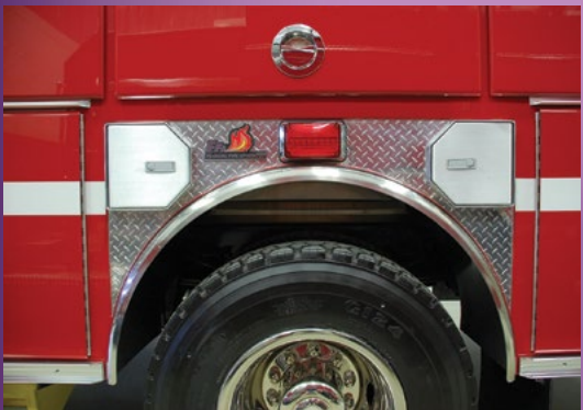
Wheel wells come standard with bright aluminum diamond plate trim, bolt in wheel well liners and polished stainless steel fenderettes.
