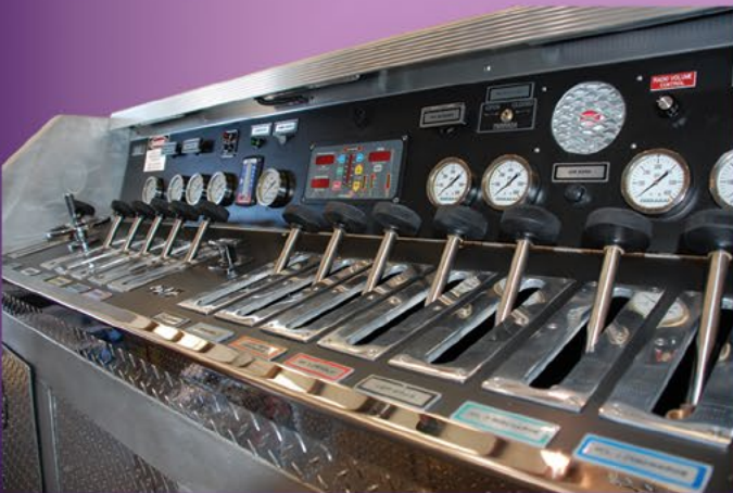
Top mount panels have a full width, hinged gauge panel. Control handle openings are finished with highly polished trim plates.
