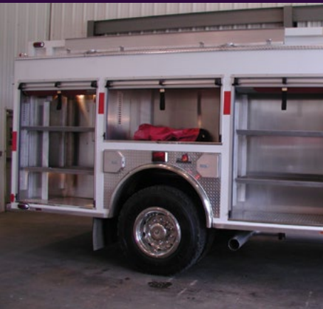
Optionally, you can get pumper compartments in a full height/full depth configuration. Standard depth is 25", with available 28" depth!
