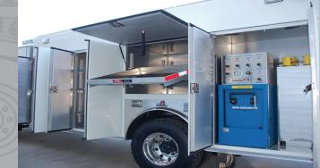
From simple SCBA bottle storage to complete compressor system with fully enclosed fill station are available on Ferrara Rescues.
