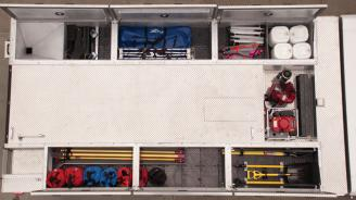
Special compartments located on the roof of the body can be designed to store additional equipment that may make the difference in a response.
