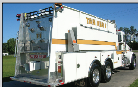
Hydraulically operated folding tank compartment
