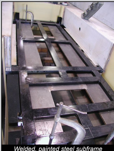
Welded, painted steel subframe
