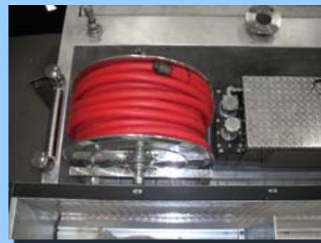
Booster Reel Over Pump
