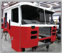
Generous door openings, low step heights and an average of 28" elbow room, make the Ultra a comfortable, easy to use cab.
