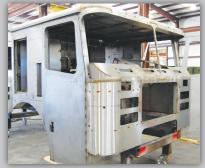
With the Ultra, we combine our legendary heavy duty construction with a rugged all stainless steel tilt cab. The Ultra cab seats crews of 2 or larger. Maintenance is easy with the Ultra's split tilt design. No need to have the crew take all their equipment out of the rear cab before tilting!
